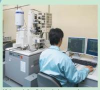
High-resolution field emission scanning electron microscope
