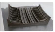
Example of molding by 3D printing: Tire mold
