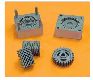
[Examples of moldings by additive manufacturing]
