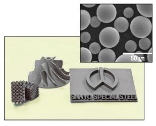
■Top: Extremely spherical metal powder (electron microscope image) Lower: Examples of moldings by 3D printing
